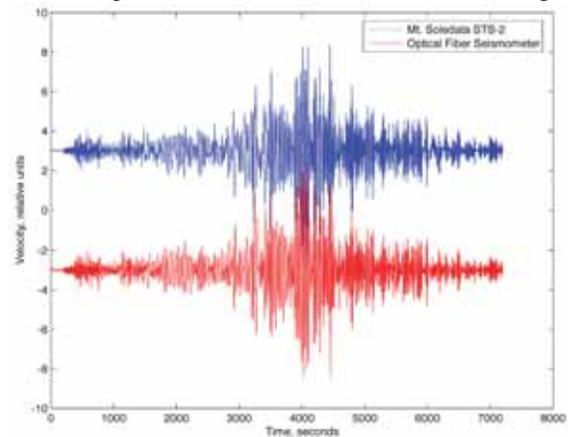
Figure 3. The 2004 Sumatra earthquake provided an opportunity to test our algorithm for converting mass displacement to ground displacement based on the spring-mass mechanical characteristics. This is a challenge because the new sensor does not rely on force-feedback as do conventional sensors. The good agreement between the record from the prototype optical sensor (red) and a conventional sensor (blue) indicates that the processing is correct (although much further work is needed).
